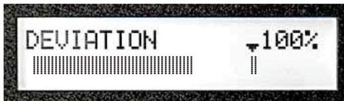
**Figure 3-13.** Press the FUNCTION Key to read Deviation
