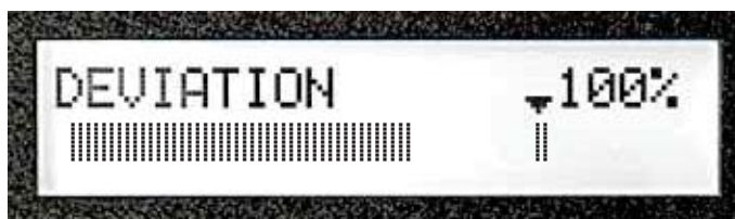
Figure 3-13. Press the FUNCTION Key to read Deviation
