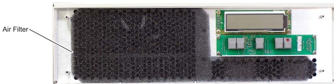
Figure 2-6. Remove the Exposed Air Filter
